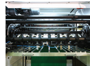
DELIVERY SECTION Sheets can be neatly stacked with side joggers.
