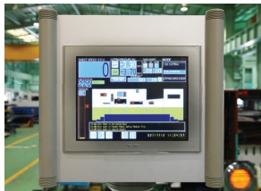
SUB TOUCH SCREEN Checks machine's condition and setting for foil adjustments.
