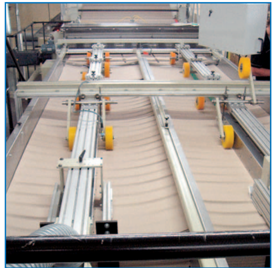
Overlapping (shingling) station for preparing the single face corrugated sheets to be delivered to the automatic non-stop down-stacker suitable for two-up production – open flute up
