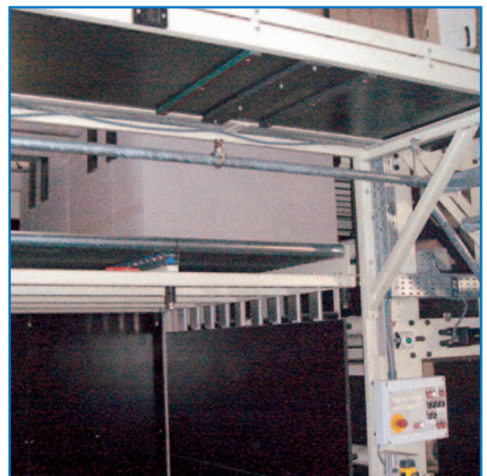
Down-stacker with non-stop operation and roller conveyor
