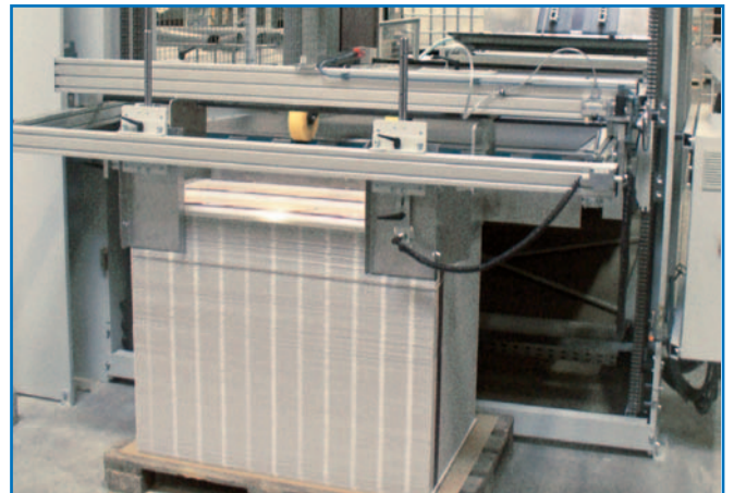
Combined pressure-belt-stacker (up-stacker): For automatic sheet delivery to a pallet with the option to take-off warped sheet batches contemporary by hand and flip them over
