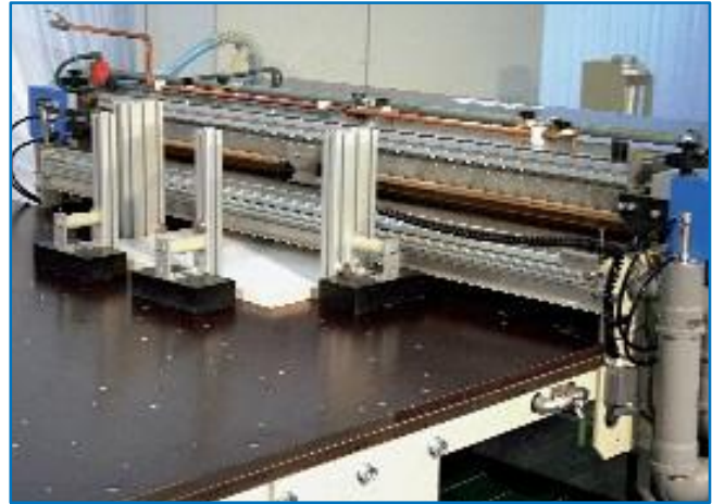
Lead edge label (printed sheet) feeder: Independent suction sleeves operate on a suction head providing fast set-up time and consistent label feeding.
