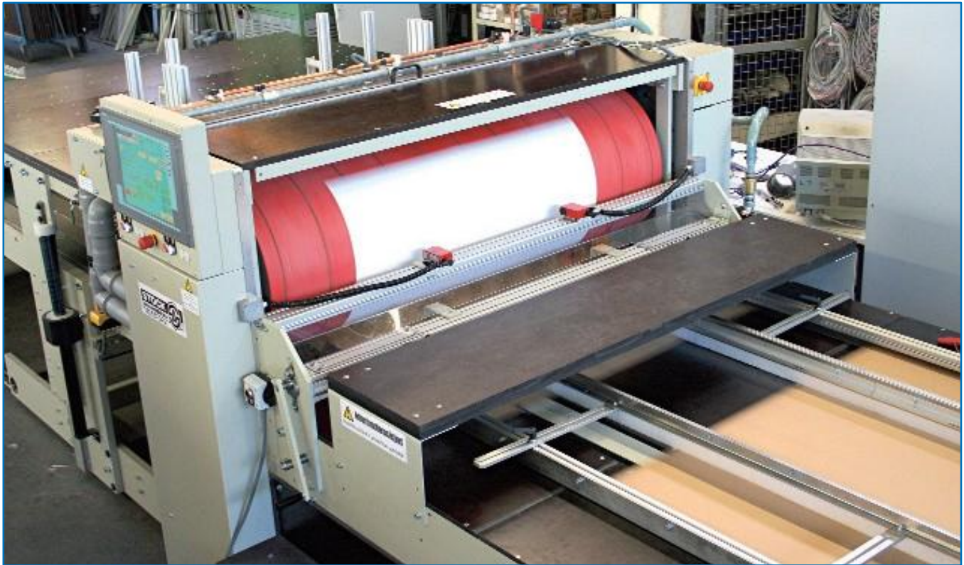
Label application cylinder: vacuum cylinder transfers the glued label to the corrugated blank, label control by laser detectors.
