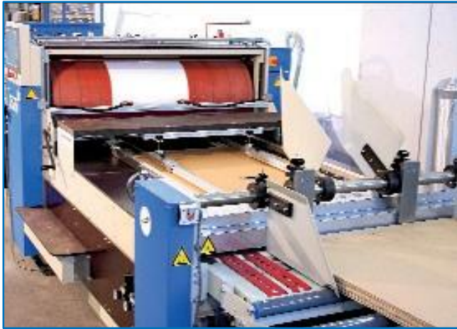
Board feeder: Lead edge suction feed. Independent driven suction belts ensure constant and accurate blank feeding.
