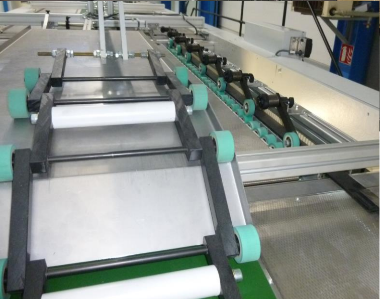
lateral adjustment of the printed sheets
