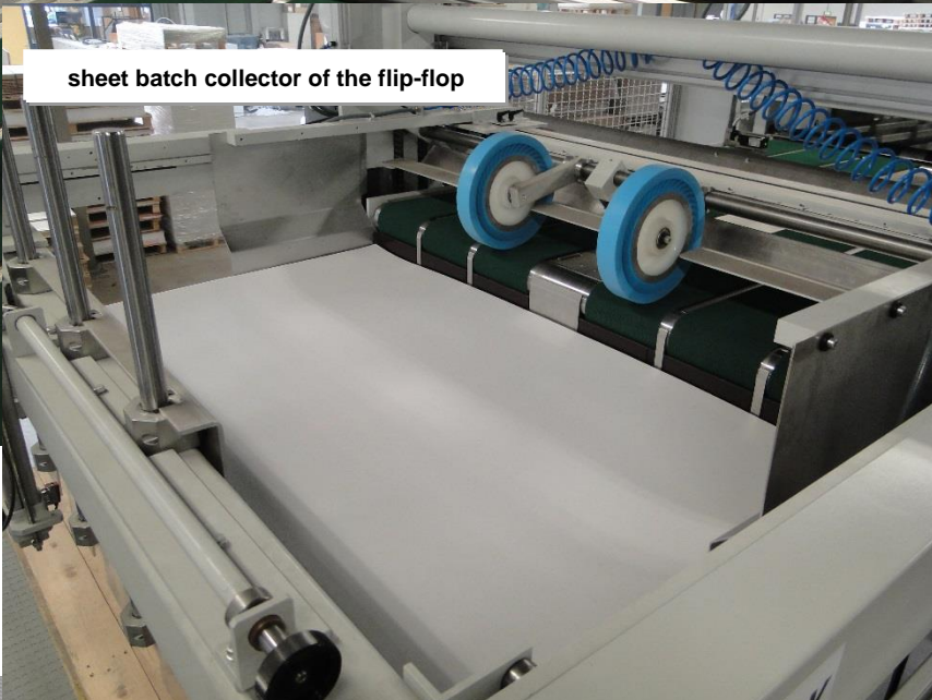
flip-flop (batch-pile turner) incl. a sheet batch collector - adjustable batch height
