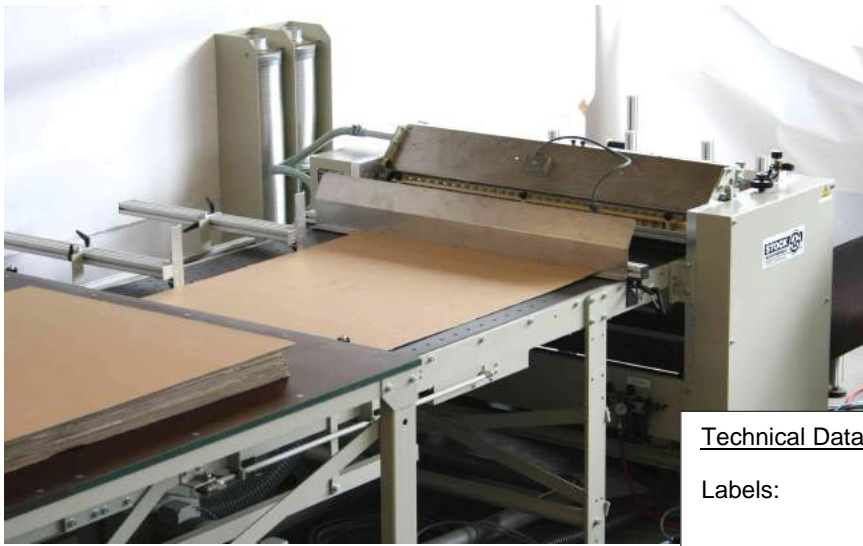
Labeling section: Manual application of the corrugated blank to the glued and placed label
