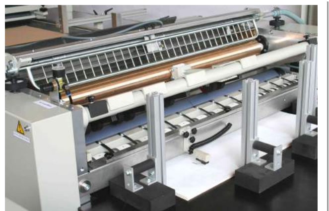
Gluing unit with pre-connected label feeder
