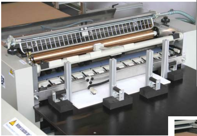
Label feeder: Single sheet feeding
