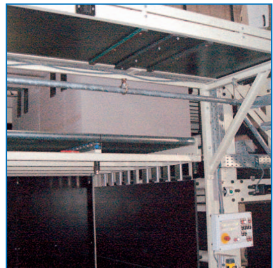
Down-stacker with non-stop operation and roller conveyor
